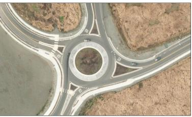
This project upgrades the compact roundabout at I-5 northbound Portal Way into a full size roundabout with slip lanes.
