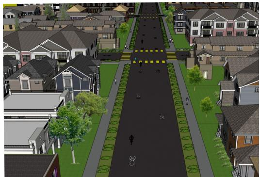
Figure 6.1.7. The medium density street design includes Sharrows (for bicyclist access on surface streets), a six-foot Bioswale, and a six-foot wide sidewalk
