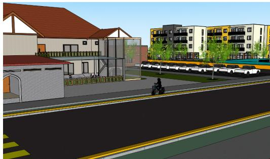
Figure 6.1.15. Street infrastructure includes a five-foot wide sidewalk, a five-foot wide bike lane, and a two-foot wide barrier for bike lane.
