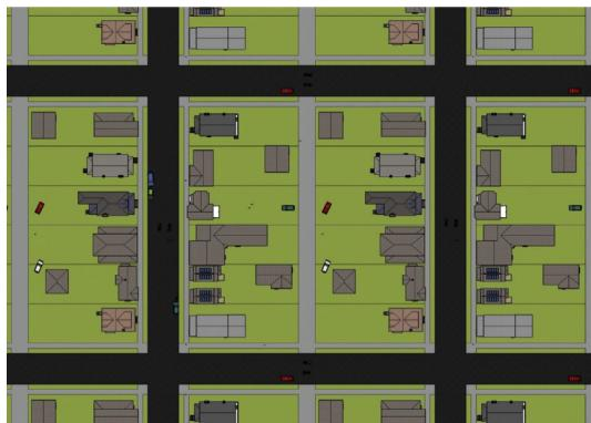
Figure 6.1.5. Site plan view of low-density zone. Bike Sharrows encourage drivers to be mindful of bicyclists and sidewalks are 6 foot widths.
